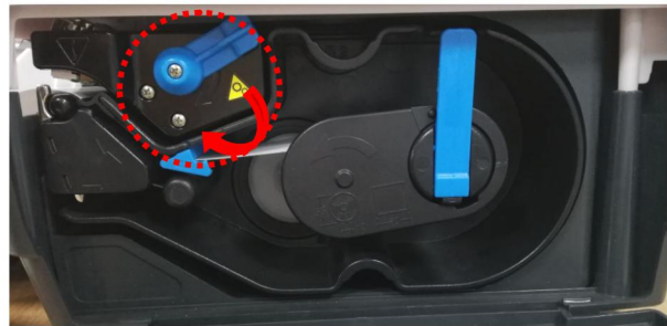
⑧ Turn lever to close position
