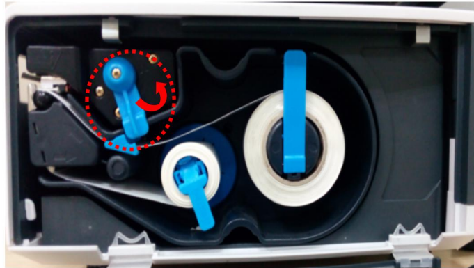
② Turn lever to open position
